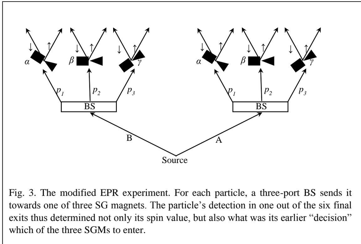
Fig. 3. The modified EPR experiment. For each particle, a three-port BS sends it towards one of three SG magnets. The particle’s detection in one out of the six final exits thus determined not only its spin value, but also what was its earlier “decision” which of the three SGMs to enter.
