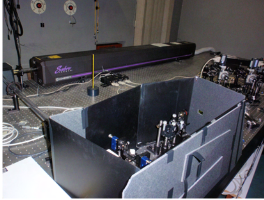
Figure 3.1 Typical set-up for Bell inequalities measurement with PDC light. In foreground one can observe the non-linear crystals where entangled photons are generated by the pump beam emitted by a laser (in background). On the right hand side the polarisation selection apparatuses and photo-detectors.
